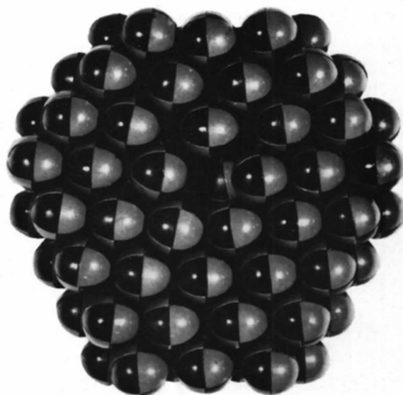
Fig. 5. A model of edge dislocation in the crystal of hexamethylenetetramine.
