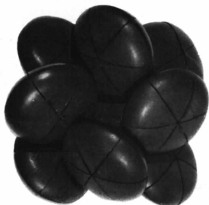
Fig. 7. Cubic Pa3 structure composed of quadrupolar oblate spheroids whose axis ratio is 2 to 1.
